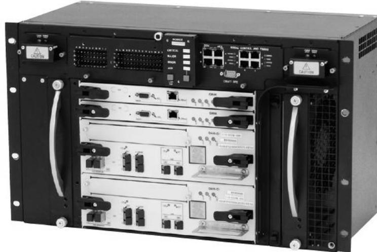
Figura 14 – Infinera Optical Line Amplifier (OLA) [27]
