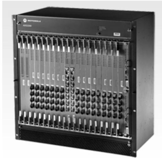
Figura 9 – Motorola AXS2200 Optical Line Terminal (OLT) [25]
